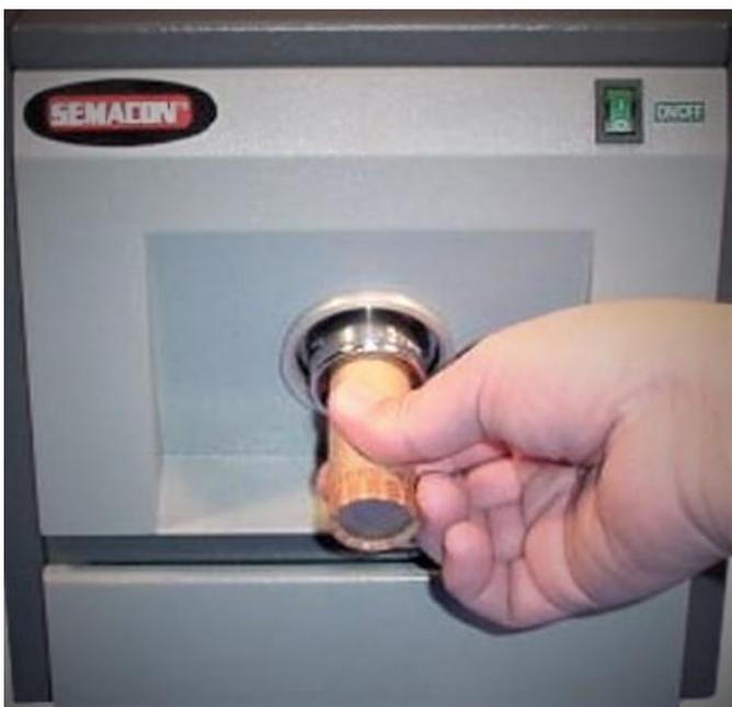
Ever wonder what makes those circular scratches on coins? The photo above shows a crimper used on the ends of coin rolls.
