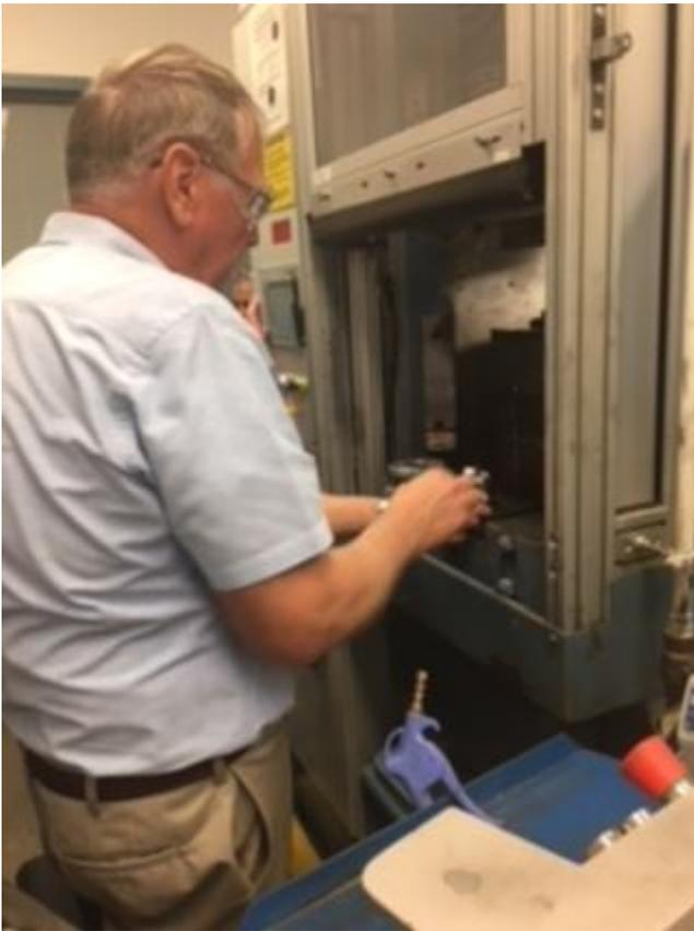
Loading a blank die into a die making machine.
